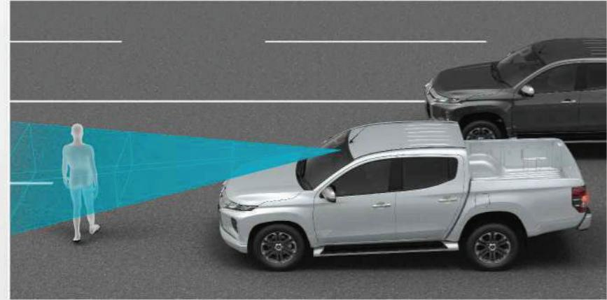
**Forward Collision Mitigation System [FCM]<sup>6</sup>**
